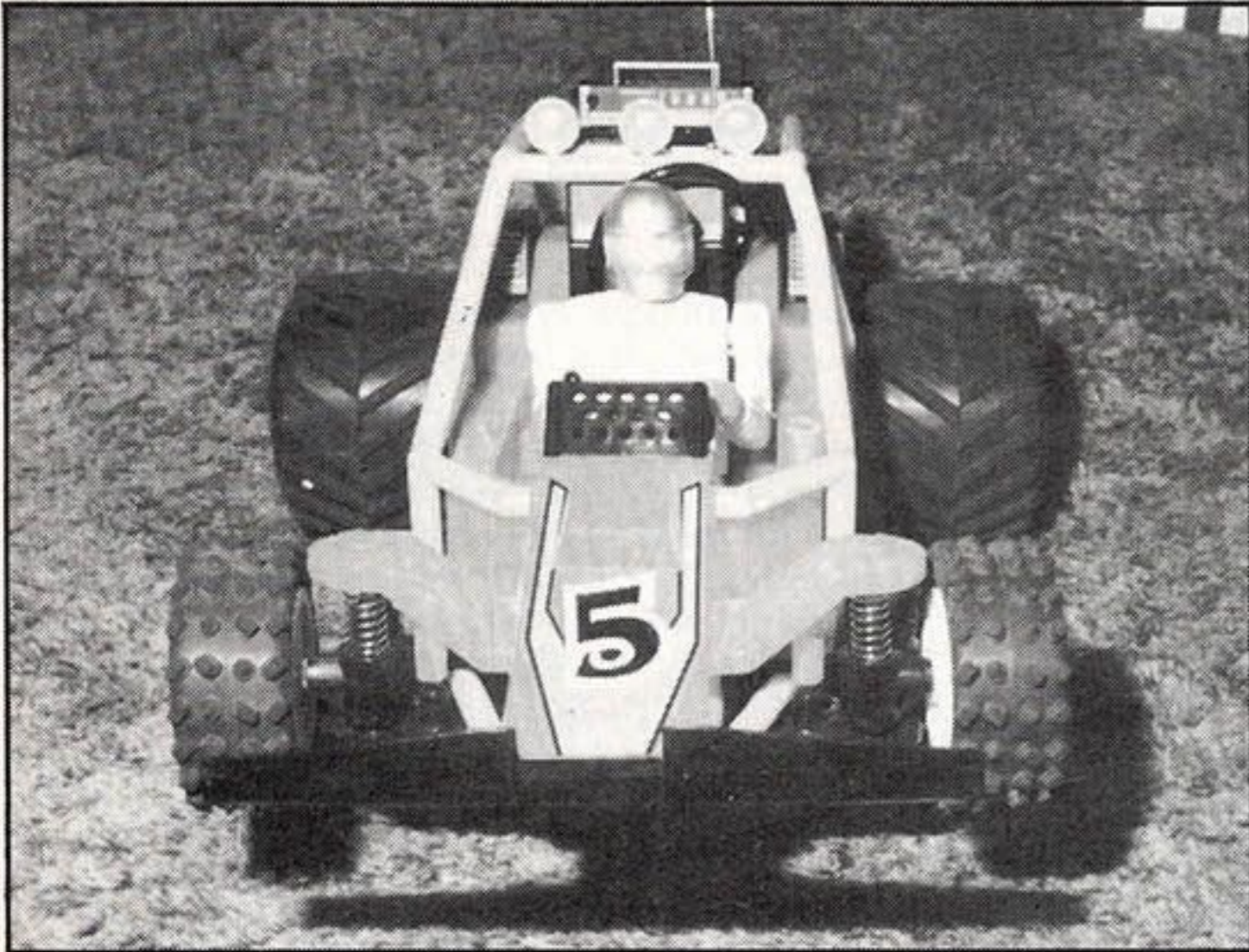
Front end is aided slightly by coil springing which works well on flat ground.
