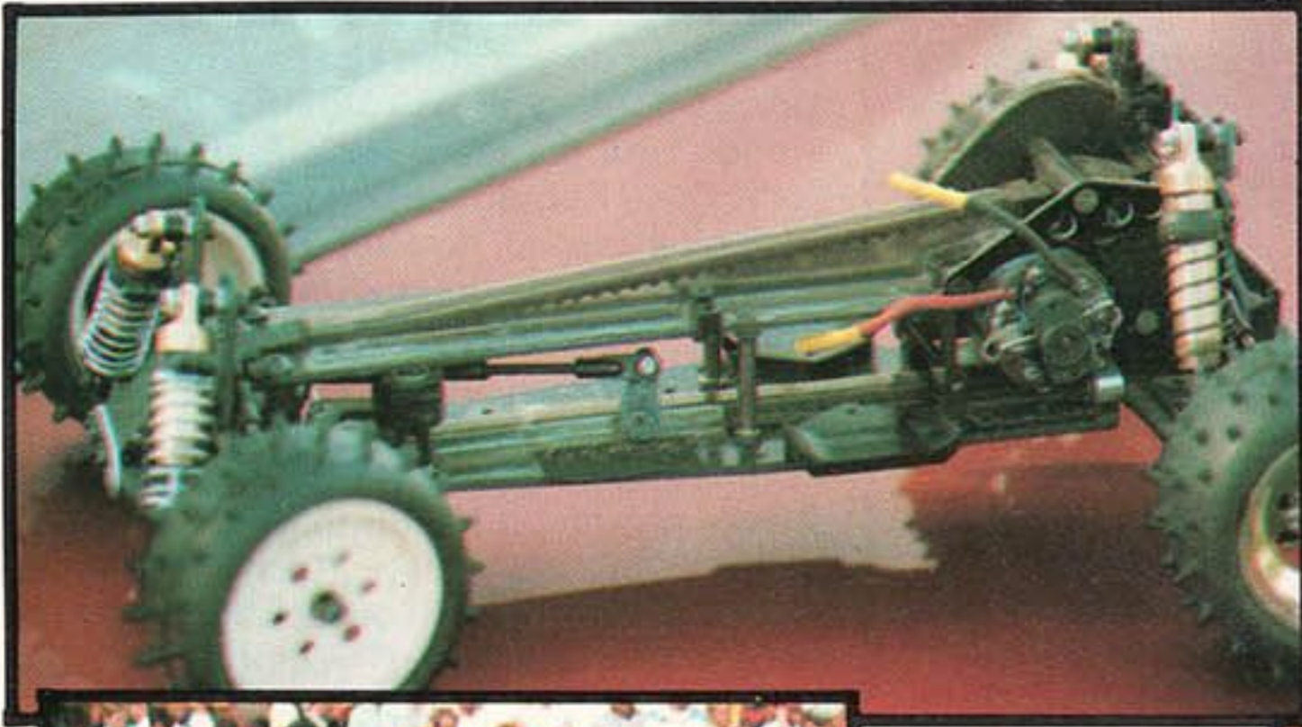
Kyosho's secret weapon the new mid engined, belt driven Optima.
